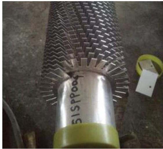
HF (high frequency) welded helical (spiral) fin tubes ( finned tubes )
