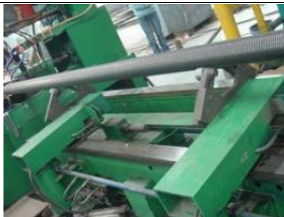
tubes (pipes) finning machines
