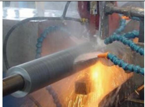
tubes (pipes) finning machines
