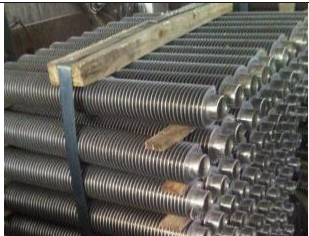
Serrated fins: HF (high frequency) welded helical (spiral) fin tubes ( finned tubes )
