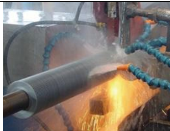
tubes (pipes) finning machines
