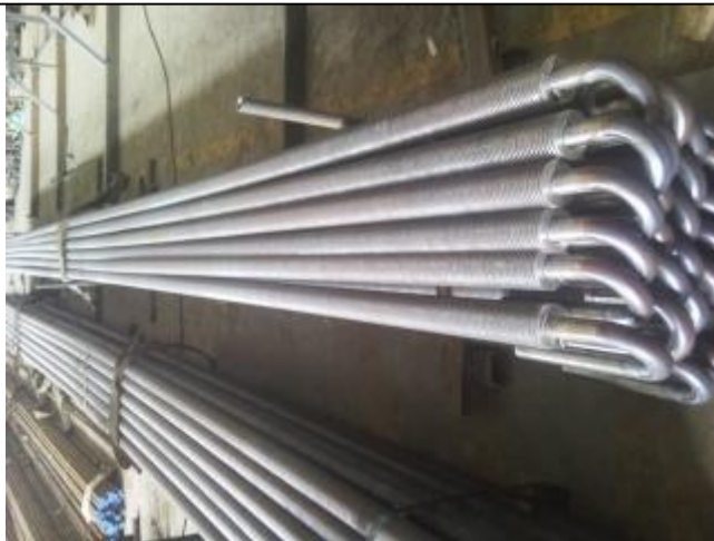
HF (high frequency) welded helical (spiral) fin tubes ( finned tubes )
