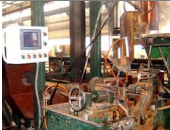
tubes (pipes) finning machines
