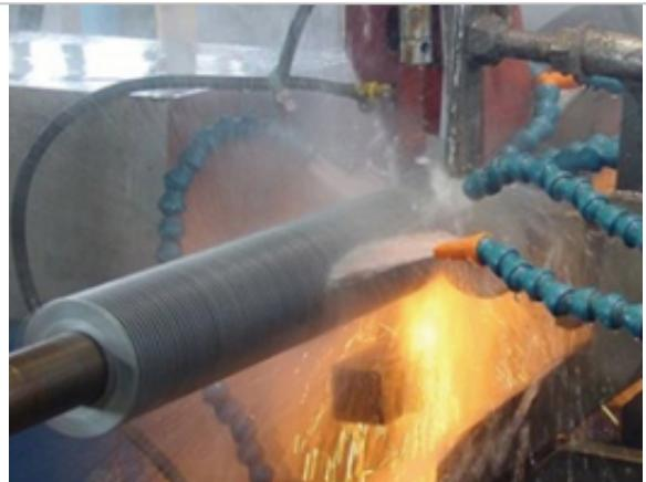
tubes (pipes) finning machines
